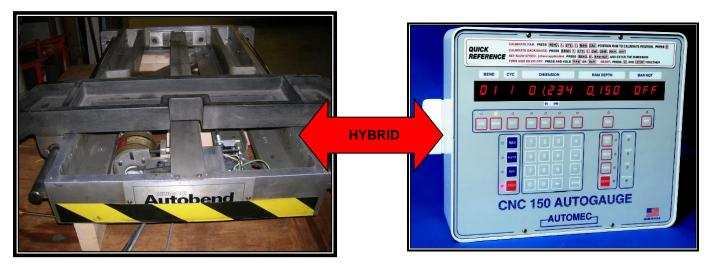
Autobend® S4 outfitted with Automec CNC150 control, encoder, servo amplifier and cables
